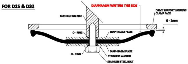
The top outer lip of the diaphragm should be 0 - 2mm from the drive support housing clamp face. To adjust the diaphragm position, loosen the lock nut at the top of the connecting rod and screw in or out as required, tighten nut once desired setting is achieved. Mount drive support /diaphragm assembly onto pump chamber ensuring the diaphragm is central and located in the groove of the pump chamber & Fit the four clamp bolts
