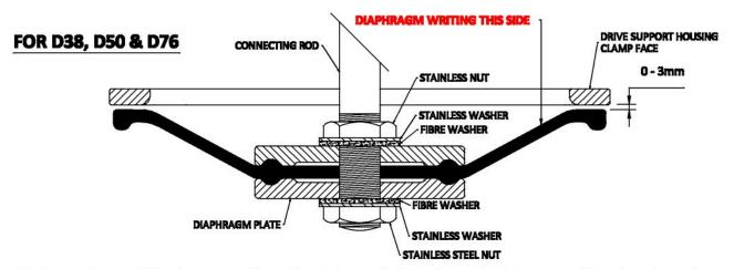
The top outer lip of the diaphragm should be between 0 - 3mm from the drive support housing clamp face. To adjust the diaphragm position, move the connecting rod nuts up or down as required. Once the correct position is achieved re-torque the bottom connecting rod nut with thread sealant to 60nm. Mount drive support /diaphragm assembly onto pump chamber ensuring the diaphragm is central and located in the pump chamber groove. Fit the four clamp bolts and torque to 25nm
